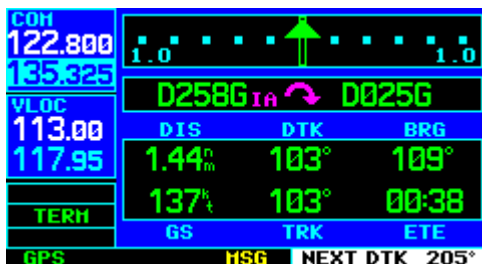
Figure 6-43 Intermediate Approach Fix
