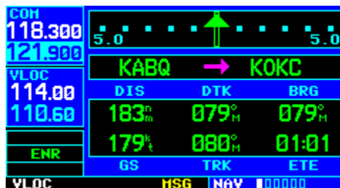
Figure 9-10 VLOC Coupled to External CDI
