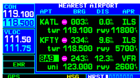
Figure 8-11 Frequency Moved to Standby Field
