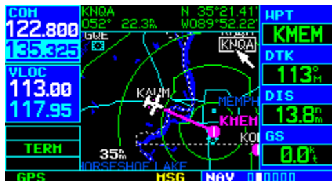
Figure 4-11 Panning Pointer Placed on Waypoint
