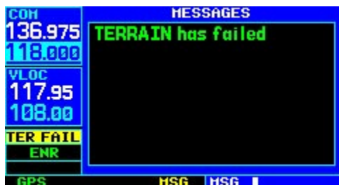
Figure 11-11 'TERRAIN has failed' Message
