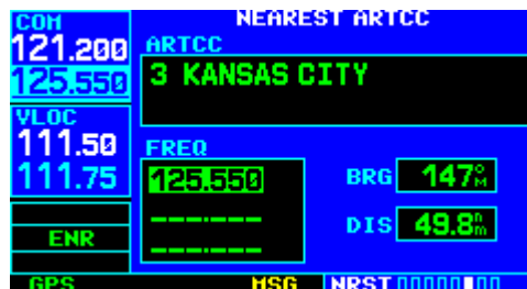
Figure 8-21 Frequency Moved to Standby Field
