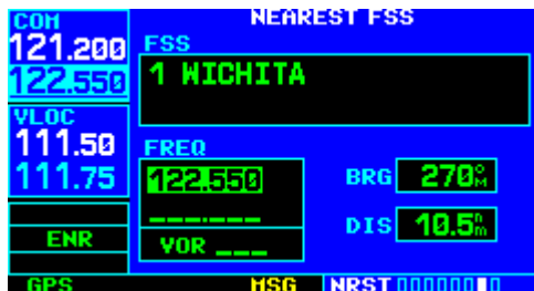
Figure 8-25 Frequency Moved to Standby Field
