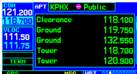
Figure 7-14 Frequency Moved to Standby Field
