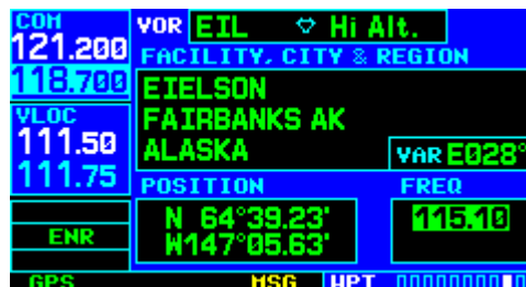
Figure 7-36 Activate the Standby Frequency
